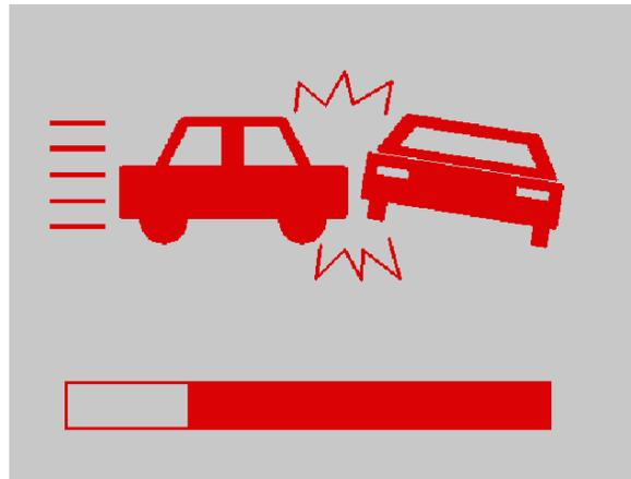
**Figure 4-5: Second warning icon option for the side mirror displays with warning icon.**
