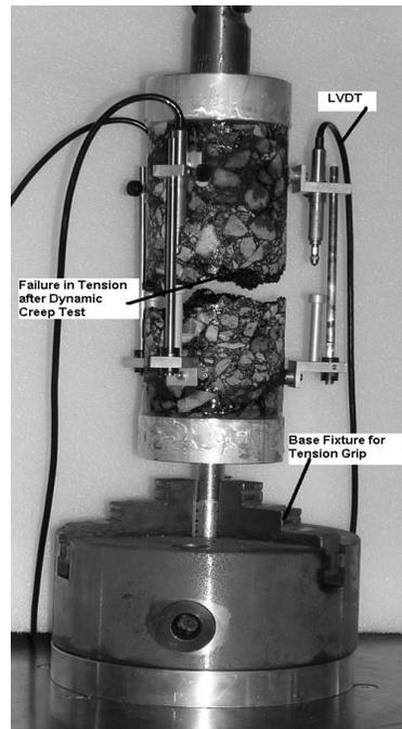
*Figure 2. Test Set Up and Sample Failure for Dynamic Creep Test (Tension)*
